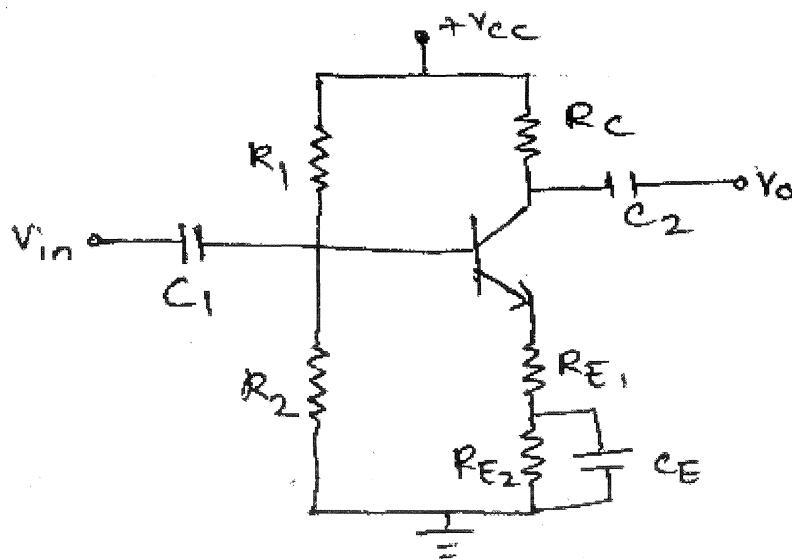
Given  $R_1 = 56\text{ K}\Omega$ ,  $R_2 = 8.2\text{ K}\Omega$ ,  $R_{E1} = R_{E2} = 750\text{ }\Omega$
